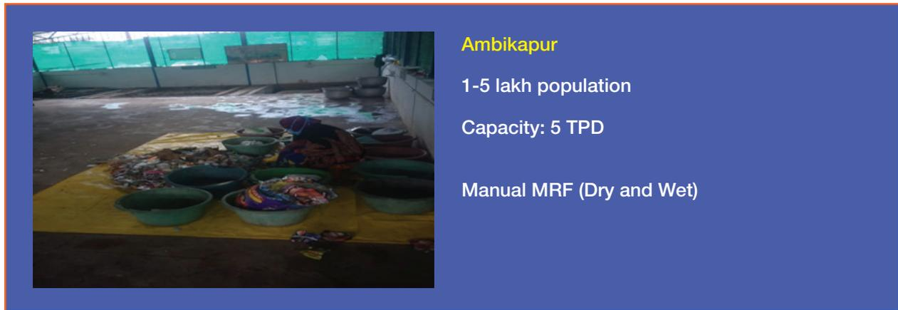
The source segregated waste is directly collected from the households by the workers in compartmentalized tricycles and taken to the facility. At the facility, secondary segregation takes place into 20 inorganic categories (paper, plastic, etc.). This followed by baling, packing, weighing and subsequent record keeping. Recyclables are sold and non-recyclables are compressed and sold for use as RDF.
