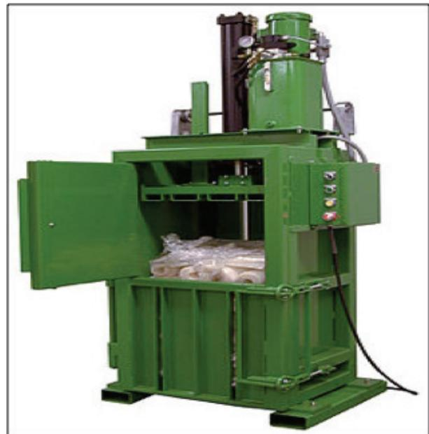
down into a dense cube, it is tied as a bale by a thick wire and then pushed out of the machine. This process allows for easy transport of all materials involved.
