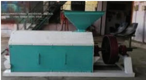
shredders tear up the plastic into small pieces/flakes, preparing them for recycling into other products. Shredded plastic is easier to use in road construction and is the feed/raw material for the agglomeration stage. Shredder includes cutting tools welded on the shaft, connected to an AC Motor.
